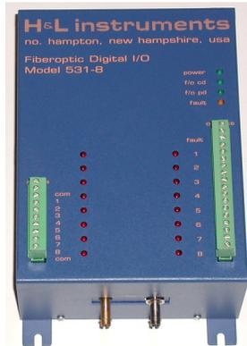
For point-to-point transfer-trip relaying, use the H&L Model 531-8 Fiberoptic Digital I/O
