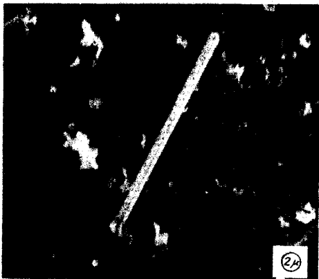
Fig. 11 Accelerated Whisker Growth. Whisker formed overnight on tin finish using procedure of Politycki and Kehren. Substrate is copper.
