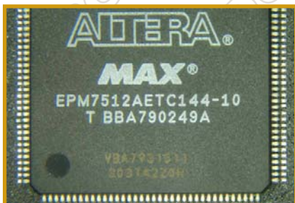
FIGURE 2: Typical quad flat pack with 250-micron gap between lead-frame tabs.
