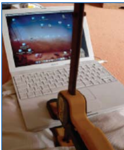
Figure 2. 'Unique' temporary repair method to press solder joint fracture surfaces together - yes, this is a C-clamp [11] .
