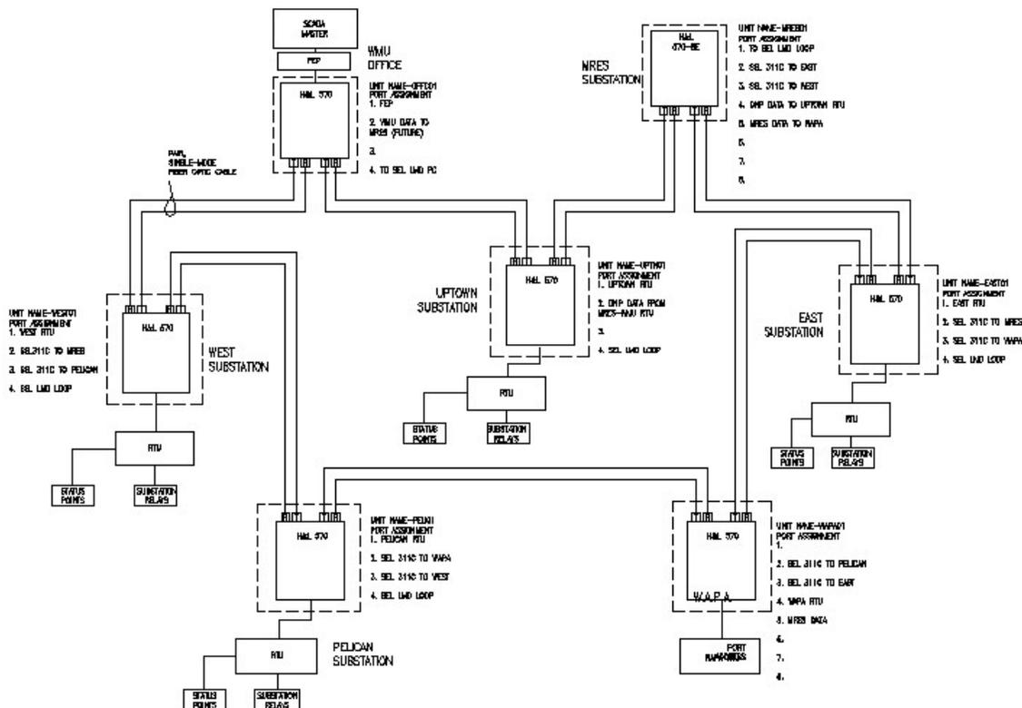
Figure 2, WMU Fiber Loop Topology
