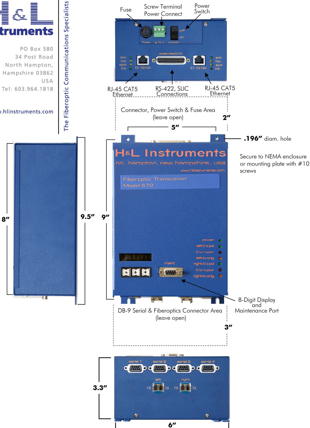
**Model 570E/570E-8 Fiberoptic Transceiver Dimensions—Standard Case**
