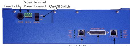
RJ-45 CAT5 Ardax, RS-422, RJ-45 CAT5 Ethernet SLIC Connect Ethernet
