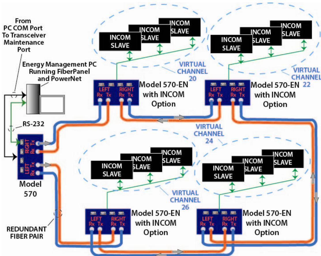
Redundant Network Solution Implements Large Networks With INCOM Support
